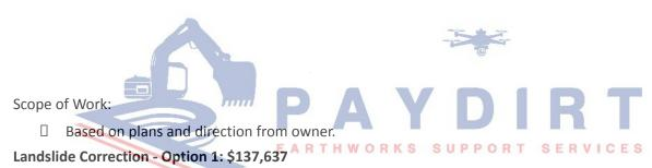
Correction of 150' L X 25' W area on hillside. Scrape of organic materials of approximately 75 CYU, import of 820 CYU of structural fill to create a 3:1 slope. Adding rip rap boulders at the bottom and 1' thick of rip rap along the whole work area, approximately 200 tons of rip rap imported. Fabric underlayment separating fill and rip rap.
